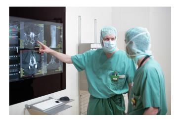
Both systems use special LCD monitors with 1920 x 1080 full HD, DICOM preset, and a 1000:1 contrast ratio. The luminance of the larger display is  $700 \text{ cd/m}^2$ , and  $250 \text{ cd/m}^2$  for the smaller display. This makes it both easy on the eyes and possible to view even the smallest of details.
